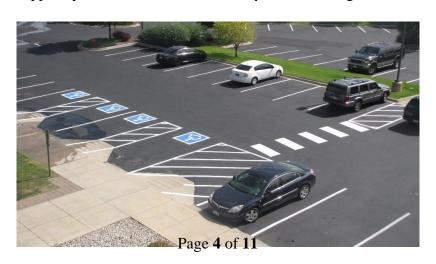
• Painted crosswalks are also required for internal sidewalks across driveways, & repainted when faded.
